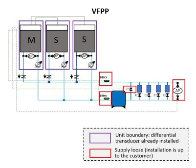
It is obligatory for the option to be combined with the Flowzer VP (inverter) and with one of the hydraulic modules that can be selected for the unit.
