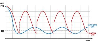
Normally, the capacity supplied by the unit exceeds the capacity actually required by the system.
