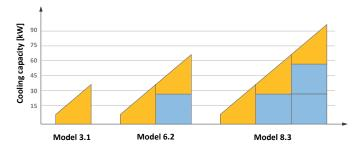
The controller uses the ON/OFF compressors to come near the required load, and modulates the capacity of the inverter compressor in order to carry out fine control.
