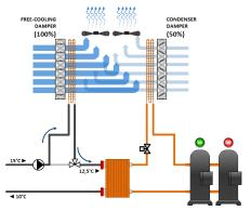
The controller switches over the 3-way valve to put the free cooling coil in series with the evaporator, fully opens the free cooling damper and pushes the fans to maximum speed. In this way, extraction of maximum cooling capacity from the outside air is ensured.
