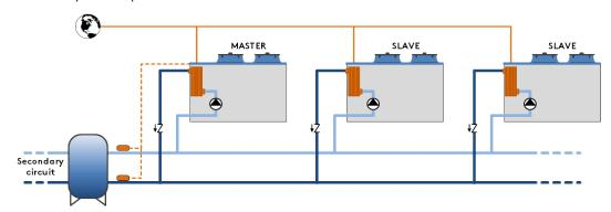
On the basis of the information recorded by the temperature probes installed on the delivery and return manifolds of the system, with the master unit, a capacity request is generated that is distributed among the units connected in the Multilogic network according to settable priority and optimization logics.
