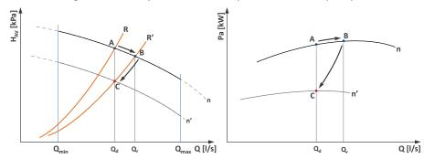
The use of the Flowzer VP allows the pump speed to be set manually (e.g. at speed n' instead of n) to obtain the design water flow rate and thermal gradient (point C). Once the adjustment procedure has been carried out, the pump will always work at a fixed flow rate.
