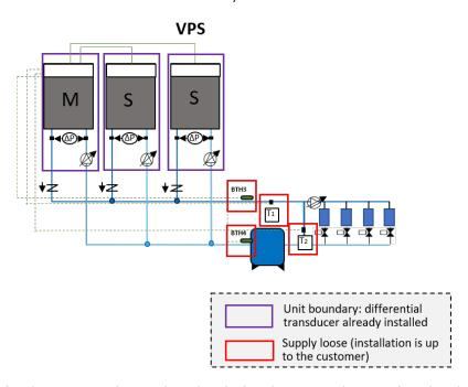
It is obligatory for the option to be combined with the Flowzer VP (inverter) and with one of the hydraulic modules that can be selected for the unit.
