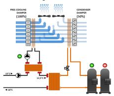
The controller switches on the circulation pump of the free cooling circuit, fully opens the free cooling damper and pushes the fans to maximum speed. In this way, extraction of maximum cooling capacity from the outside air is ensured.
