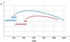
It can also be seen that, since it is specially built to also operate at low speeds, a BLDC compressor has a wider speed adjustment range than a conventional compressor controlled through an AC inverter.
