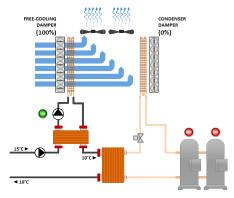
The capacity given by the water coil fully meets the requirement of the system, and therefore the damper in front of the condenser is fully closed and the compressors are kept switched off.
