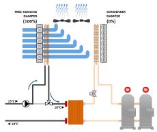
The capacity given by the water coil fully meets the requirement of the system, and therefore the damper in front of the condenser is fully closed and the compressors are kept switched off.
