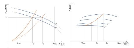
This accessory is useful when the total head losses of the circuit are slightly variable or when they change depending on the seasons (for example, some user points are active only during summer operation and not during winter operation).
