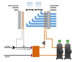
In this mode, the damper that controls the air flow rate at the free cooling coil is fully closed, whereas the one in front of the condensing coil is fully open. The 3-way valve bypasses the free cooling coil (to prevent unnecessary head losses) and condensation control is done, when necessary, through modulation of the fans.
