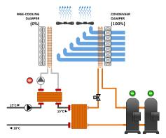
In this mode, the damper that controls the flow rate at the free cooling coil is fully closed, whereas the one in front of the condensing coil is fully open.
